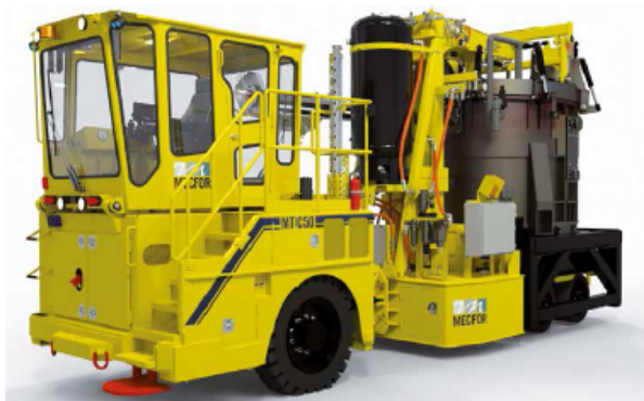
The Mecfor MTE50 Crucible Hauler syphoning tube remains wholly immersed in the molten metal during transfer.
