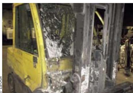
**Metal splash on industrial forklift while loading ingot into furnace. The forklift gets too close to the furnace sill.**
