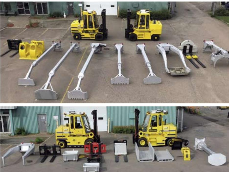
Mecfor casthouse solution with QuicConnect charging and tending tools for various tasks
