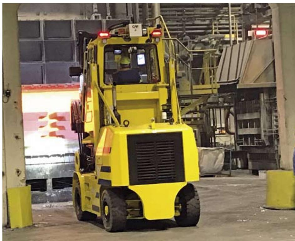
**MVR22 with lifting cab**
